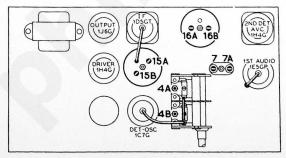
Fig. 2. Locations of Compensators-Top of Chassis
