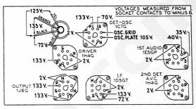
Fig. 1. Socket Voltages, Underside of Chassis
